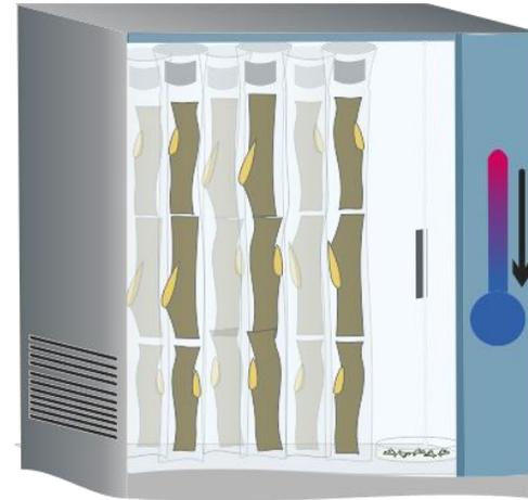
Cooling rate at  $1^{\circ}\text{C h}^{-1}$
