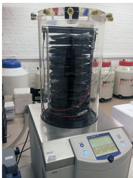
Freeze-drying device for leaf samples
